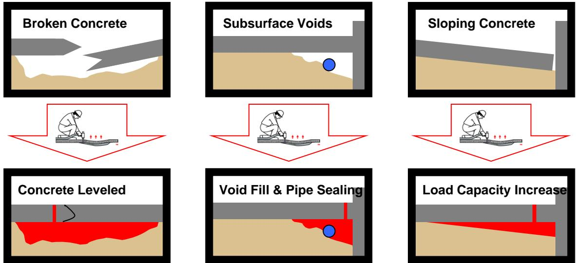
The **Uretek Method** utilizes the most advanced technologies and injection techniques in the industry. Using the most dense polymers in available, the patented Uretek 486 polyurethane foam is injected into voids or under concrete, via 5/8" holes. The material expands at a 100% predictable rate of 20:1, allowing for the most accurate re-grade and slab alignment in the industry. And, reaching 90% strength in 15 minutes means that you get 'back to business' almost immediately.
