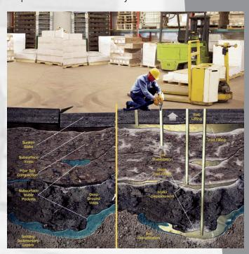
In areas where there are no significant voids the concrete will begin to lift immediately, resulting in a reduction of material consumption. The URETEK material offers the benefits of significantly increasing load bearing properties of the fill and sub-base, long term stability, thermal insulation and moisture sealing.
